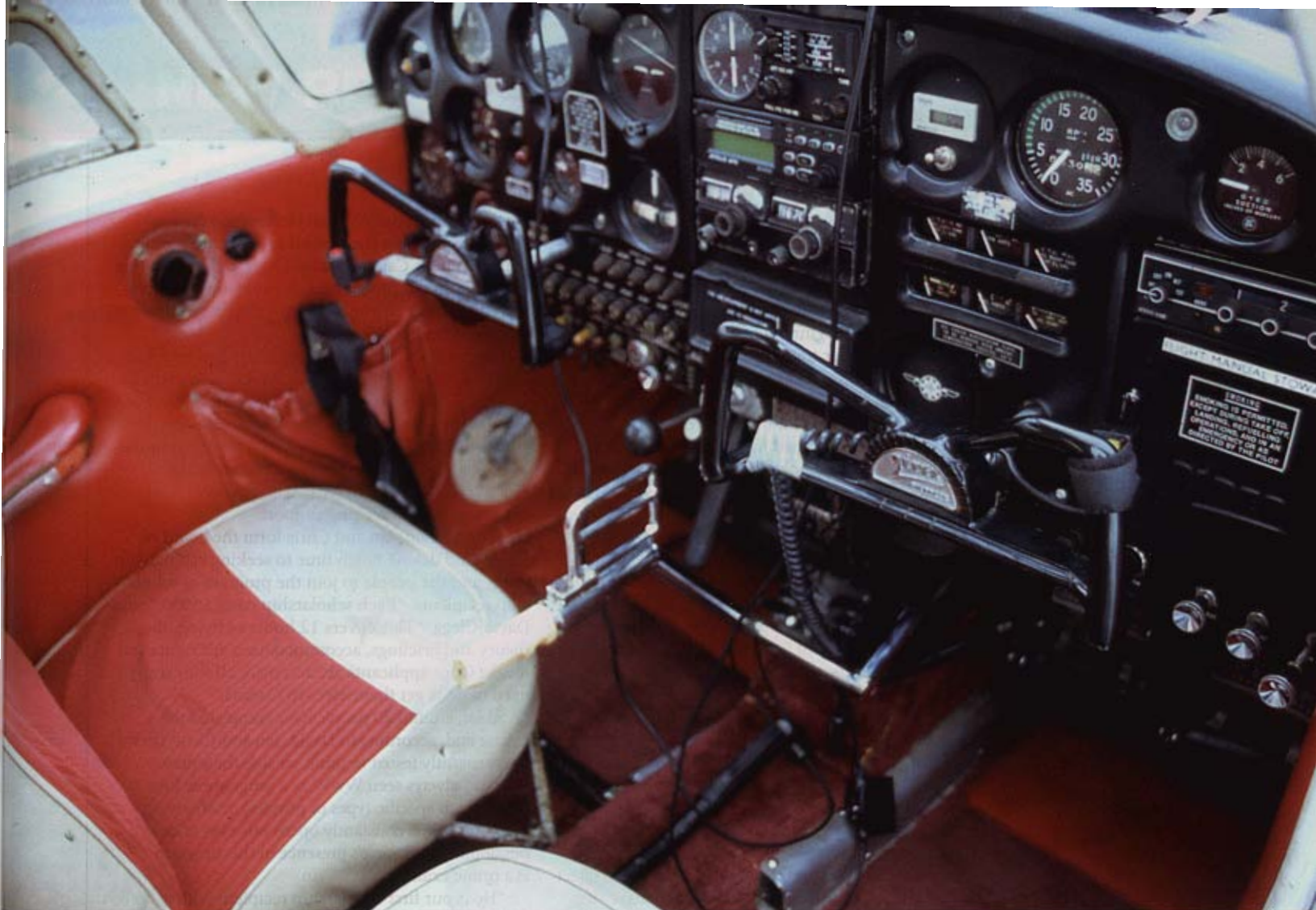
Above: The cockpit of the Piper Cherokee 140 used to train WwW's students, showing the hand control installed.
